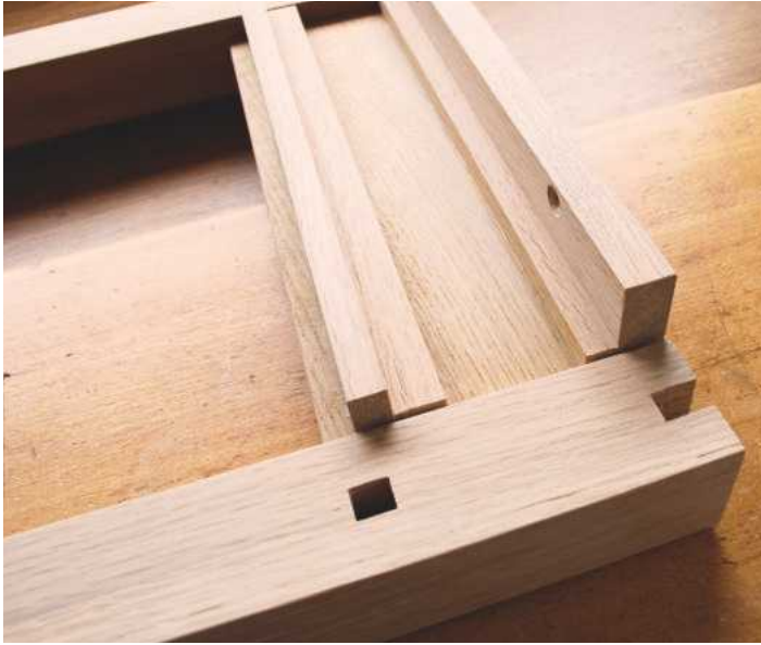
▲ Pic.3 The drawer runners and kickers, made from rebated oak, are glued to the insides of the side rails
